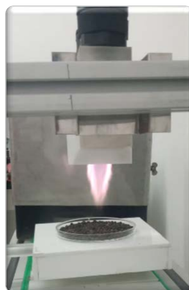
Atmospheric Pressure Gliding Arc Discharge Cold Plasma equipment (APGADCP)
