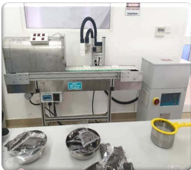
Atmospheric Pressure Gliding Arc Discharge Cold Plasma equipment (APGADCP)
